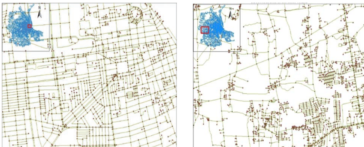
Figure 5.2. (Left) the street networks in the inner Khans and (Right) the street networks in suburban Khans. Red dots represent the nodes and cul-de-sacs, and the light green represents the edges (Research Team, 2020)
